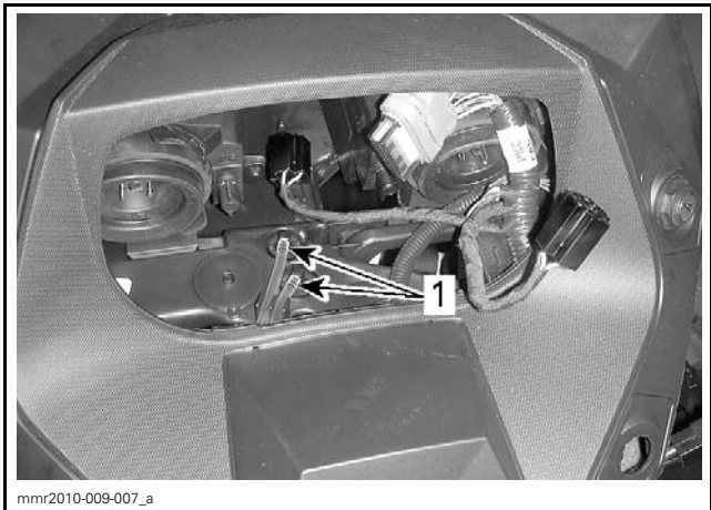
TYPICAL 1. Carburetor vent tubes
